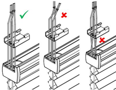
For child safety, please check and ensure that there are no loose cords after the shade is completely installed. If the shade is too loose, please retie a new knot for it. Remove bottom shoe slider, untie the knot and make a new knot for adjustment. Please do not tie the cord too tight as it will cause too much friction.
