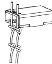
Notes: When installing the Shoe slider, it is suggested to secure the bottom shoe slider first, and then unfasten the top cord to secure the top shoe slider. Please do NOT untie the top cord until the bottom shoe slider is secured.
