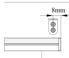
Make sure to keep minimum distance (L2) between the edge of L bracket and the top/bottom window frame ≥9mm.
