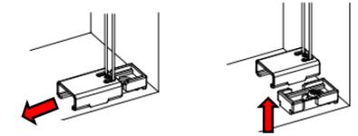
a. The light guard is to be placed at back or front of the shade at left & right side.
