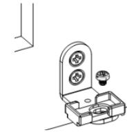
For shade width reaches 1270mm with center cord, after installing L bracket at the ends, install two L brackets in the center at top and one L bracket in the center at bottom, and keep them align with the end L brackets. The outer edge of Shoe Bases should head to the middle line, and the outer edge of the left Base should align with the middle line, as illustrated below. **The bottom Shoe Base needs to align with the left one at the top center.**
